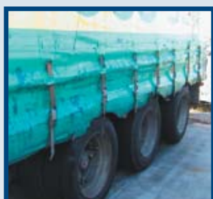
Poorly repaired curtains
