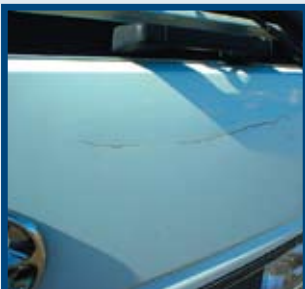
Scratches over 100mm in length that penetrate to bare metal or primer
