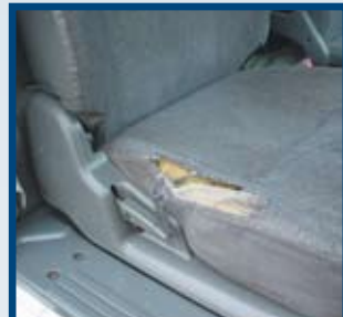
Excessive wear to seat base
