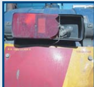
Any hole or crack in a lamp or glass lens
