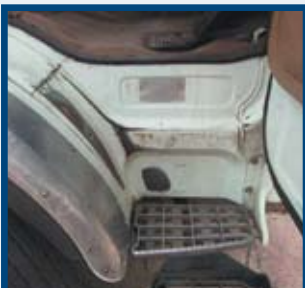
Missing or broken cab steps or step pads
