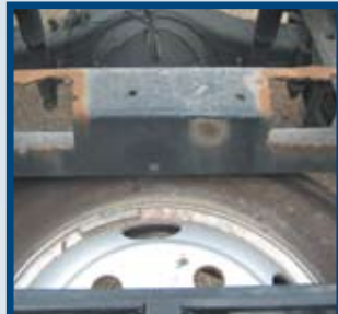
Chassis modifications without authorisation
