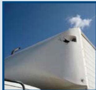
Cracking to body
