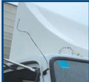
Bent, broken or missing aerials
