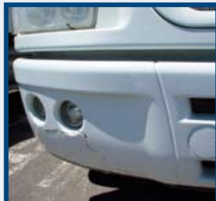
Any bumper that is incomplete, cracked, twisted or misaligned
