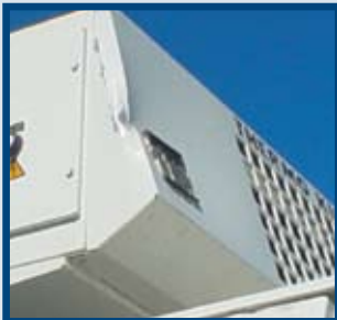
Damaged air con accessory
