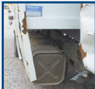
Multiple dents in a localised area that are up to 45mm in diameter
