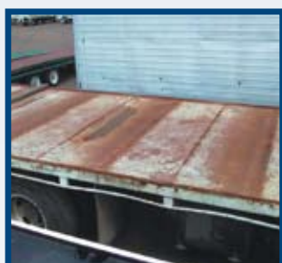
Bent or broken tie rails
