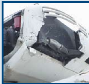
Damaged refrigeration unit
