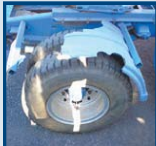
Damaged wheel guards
