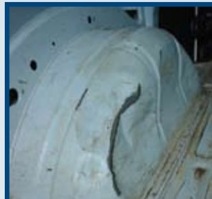
Dents over 30mm in depth or that have changed the overall shape of panelling
