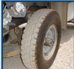
Missing wheel guards
