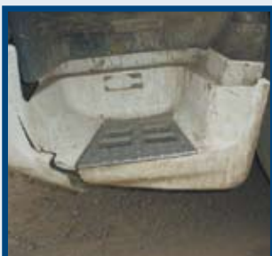
Cabin - damaged step
