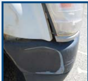
Any bumper that is incomplete, cracked, twisted or misaligned
