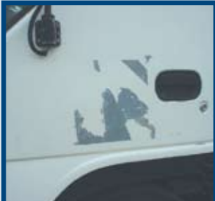
Any damage caused by the removal of signage or decals
