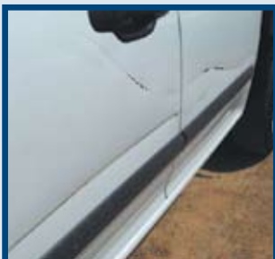
Scratches over 50mm in length that penetrate to bare metal or primer
