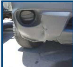
Bumper cracked and deformed
