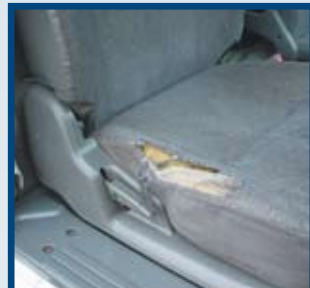
Excessive wear to seat base
