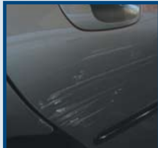
Multiple scratches in localised area where bare metal or primer is exposed
