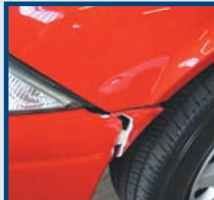
Bumpers or rubbing strips that are cracked, broken, missing or severely damaged
