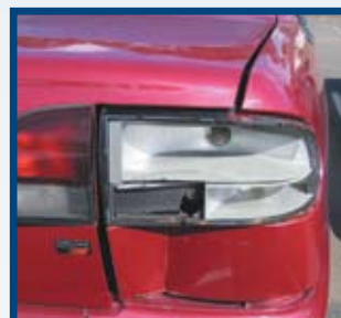
Any crack or hole in lamp glass that allows water to penetrate
