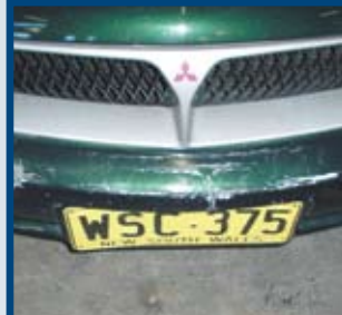
Bumper with excessive scuffing
