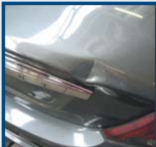
Isolated dents over 20mm in diameter
